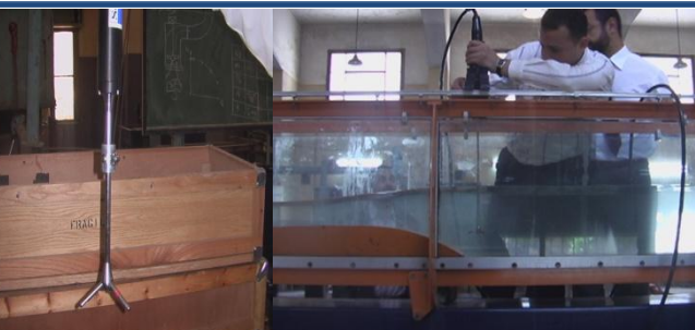
Training Engineers how to use ADV to measure turbulence
