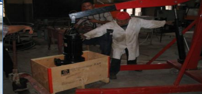
Pump Performance and Acceptance Test
